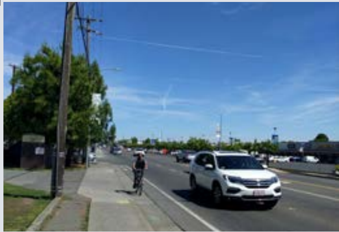
Narrow bike lanes include the gutter
